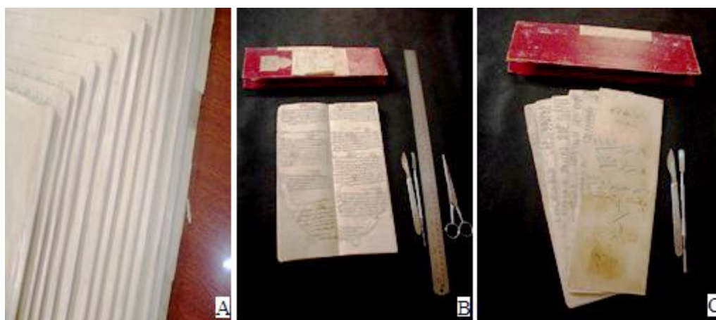
[FIGURE 16]: Finishing procedures: A- reassembling the sheets of papers together into folders; B & C- the archive folders after sewing and rebinding process.
