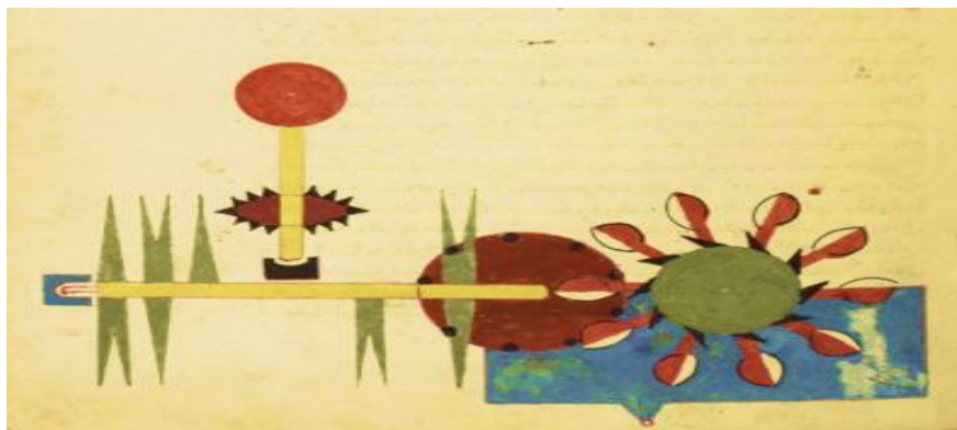
[FIGURE 6]: The cam mechanism
