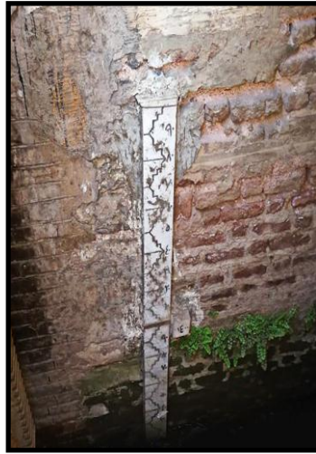
Plate No. 33: The Nilometer located at the entrance of the Sarsawiya barrage (Photographed by the researcher)
