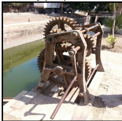
Plate No. 15: The crane used in Bagouria Lock. (Photographed by the researcher)
