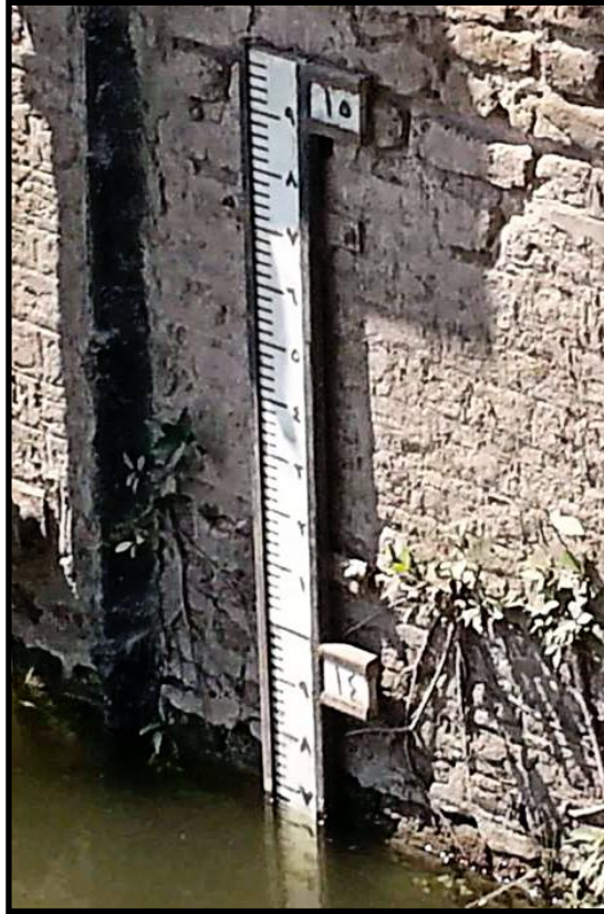
Plate No. 36: A Nilometer located at the eastern side of the front façade of the Bagouria barrage (Photographed by the researcher)
