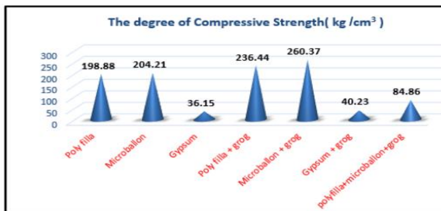
[FIGURE 6]: Represents determination of compressive strength degree of some selected filling materials
