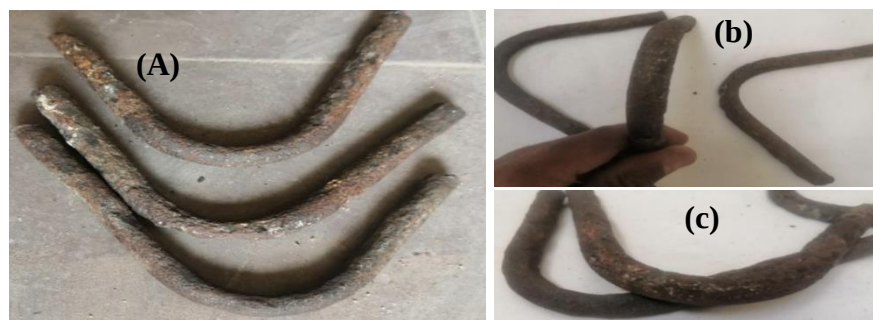
[FIGURES 9/A-C]: The results of the bending test, which showed good resistance to the bending strength and the absence of cracks. © Done by the authors
