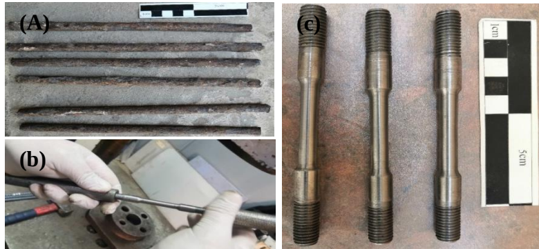
[FIGURES 3/A-C]: Preparing steel rebar samples in preparation for the tension test © Done by the authors
