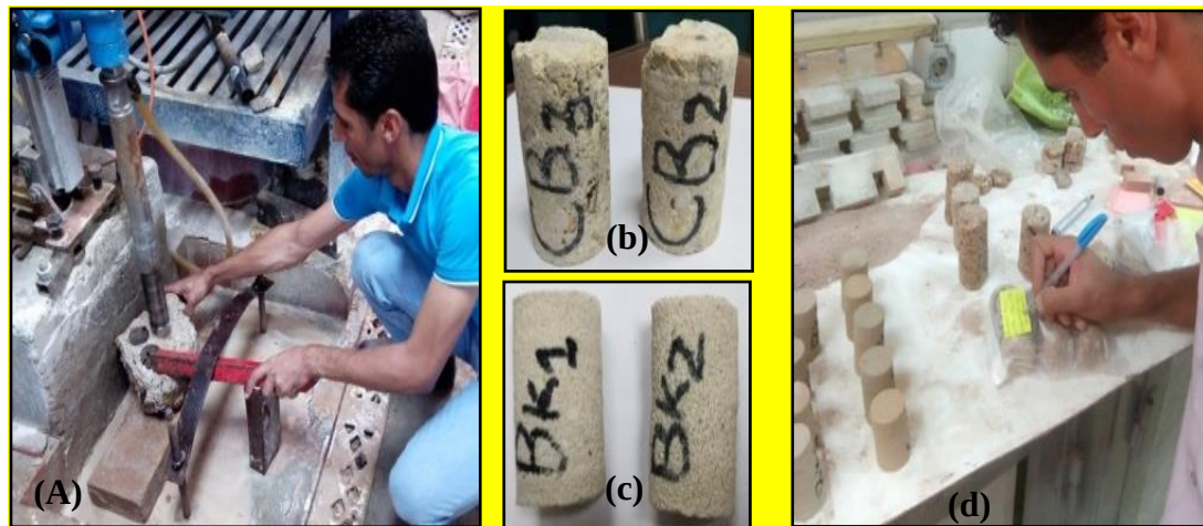
[FIGURES 1/A-D]: Preparation and coding of the building materials specimens and samples under investigation © Done by the authors.
