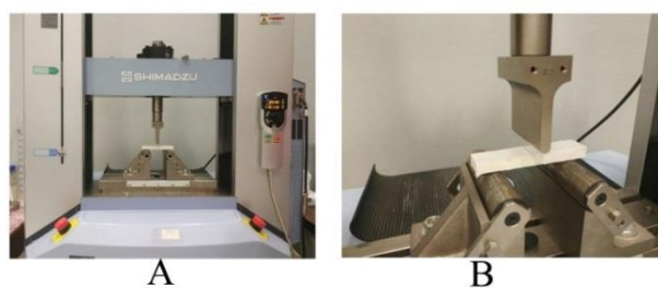
[FIGURES 15/A-B]: Shows Mechanical testing apparatus and three-point bending test method © Photo taken by OSAMA SAMIR
