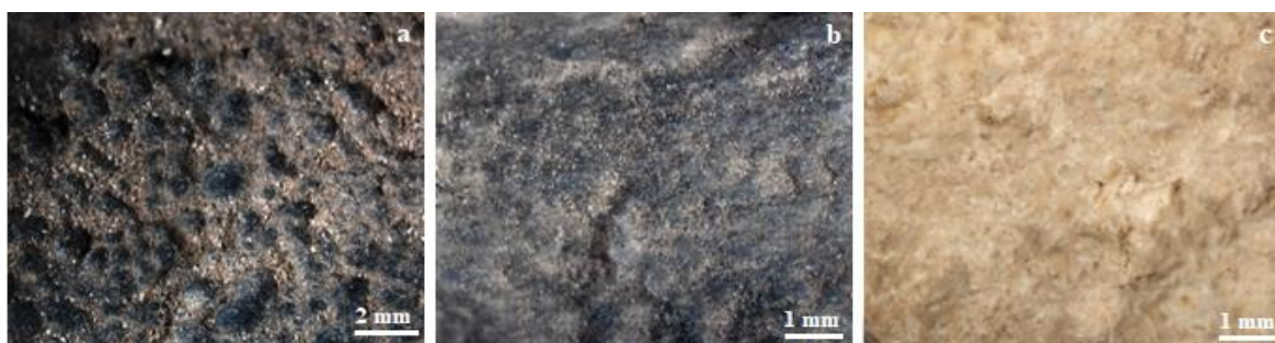
[FIGURES 5/A-C]: Stereo micrographs of a limestone [Sample N o .2]; A. Before treatment; B. After chemical pre-treatment; C. After biological treatment © Done by the researchers
