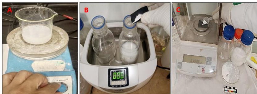
[FIGURES 5/A-C]: Different stages of preparation of the nanocomposites used in the study © Photo taken by the authors
