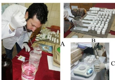
[FIGURES 14/A- C]: A. Shows Preparing an acidic sulfuric acid solution; B. Soaking samples in the acidic solution; C. Weighing samples before and after soaking in the acidic solution © Photo taken by
