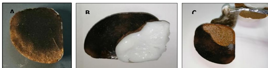
[FIGURES 1/A-C]: Visual examination before, during and after the application process, which ranged between 2-3 mins. The hydrogel was removed by forceps as a cohesive unit. The cleaning efficacy of the soot stain with no residues observed on the surface © Done by the authors
