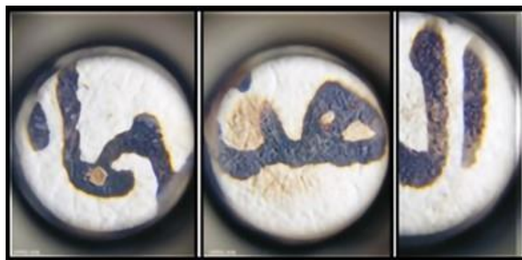
[FIGURE 7]: Iron ink corrosion observed using a smartphone microscope (OPPO 16), showing brown spots, paper staining and ink fading © Photo taken by AHMED HOSNI
