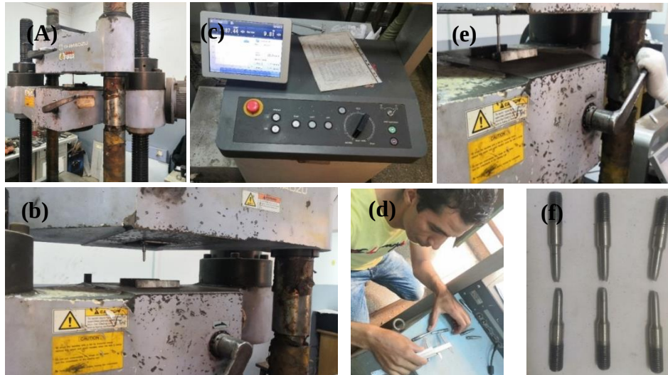
[FIGURES 4/A-F]: Setting steel rebar samples in the test device and conducting the tension test © Done by the authors
