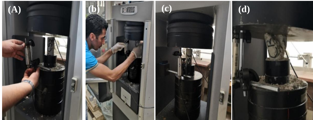
[FIGURES 2/A-D]: Uniaxial compression test setup for reinforced concrete, bricks and steel rebar © Done by the authors
